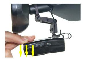
4 - To access the buttons of the RD you will need to gently push downward on the front of the RD with one finger and push the desired button with another finger. Then allow the RD to return to it's original position by gently letting it spring upward. When accessing the buttons, be sure to push the RD downward just enough for your finger to fit between the RD and mirror. Do not push down more than what is needed.
